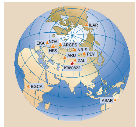
Figure 1 Azimuthal equal-area projection of the Earth, centred on the epicentre of K980822, showing the IMS stations that recorded seismic waves. Origin time, 05:00:18.94 UTC; estimated origin time, 05:00:18.7 UTC. Epicentre, 49.7667° N, 77.9908° E; estimated epicentre, 49.7566° N, 77.8273° E. Depth, 0.140 km. Firing medium, granite. Explosive, 100 tonnes of Granutoll. Estimates are from the prototype International Data Centre's Reviewed Event Bulletin . ARCES, Karasjok, Norway; ARU, Arti, Russian Federation; ASAR, Alice Springs, Australia; BGCA, Bangui, Central African Republic; EKA, Eskdalemuir, UK; HFS, Hagfors, Sweden; ILAR, Eielson, Alaska, USA; NOA, Hamar, Norway; NRIS, Norilsk, Russian Federation; PDY, Russian Federation; ZAL, Zalesovo, Russian Federation.
